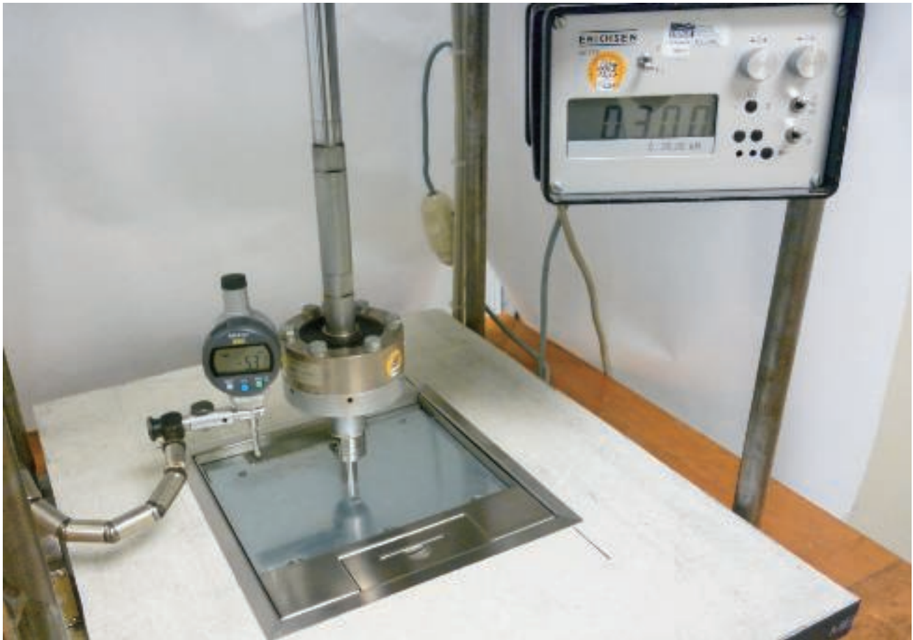
Figure 2: Load testing of a metal service outlet with 3 kN and a permitted bend of less than 6 mm
