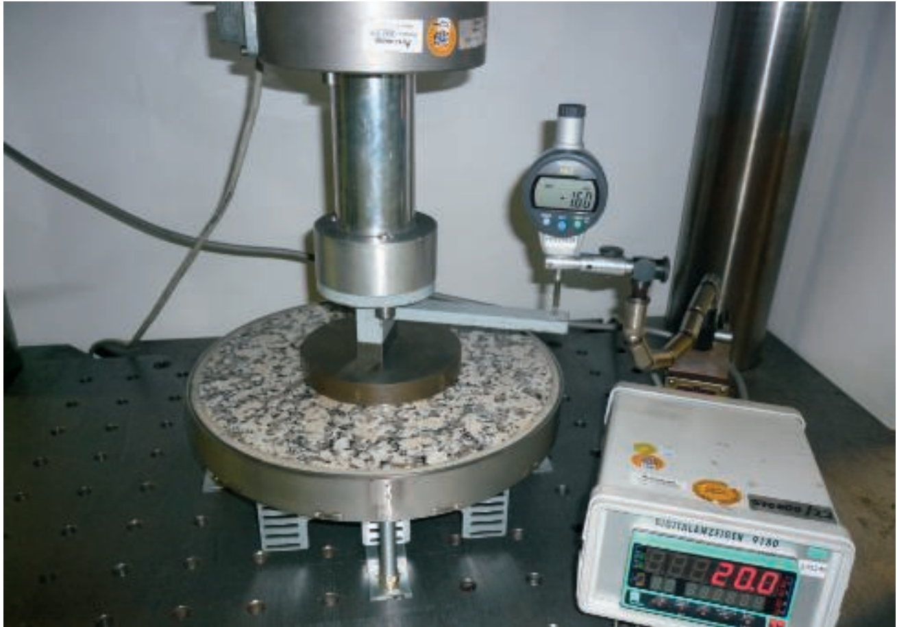
Figure 1: Load testing of a heavy-duty cassette with 20 kN
